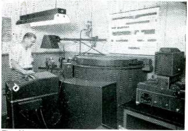
This Mallory spectrographic device tests the purity of metals and alloys.
