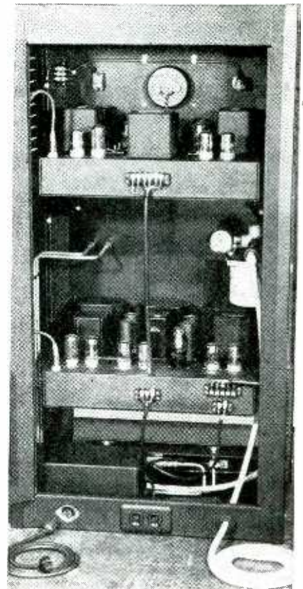
Rear view of gyro balancer, showing how amplifiers are arranged on two separate chassis units that can readily be removed for servicing
