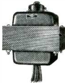
Mounting type 150. 4 hole horizontal mounting. Lead holes on bottom or side of shell. Primary tap changer on top. Ratings 35 to 500 VA.
