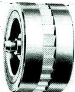
FIG. 1—Gyro rotor. Air stream impinging on vanes in center drives rotor at 12,000 rpm during balancing tests
