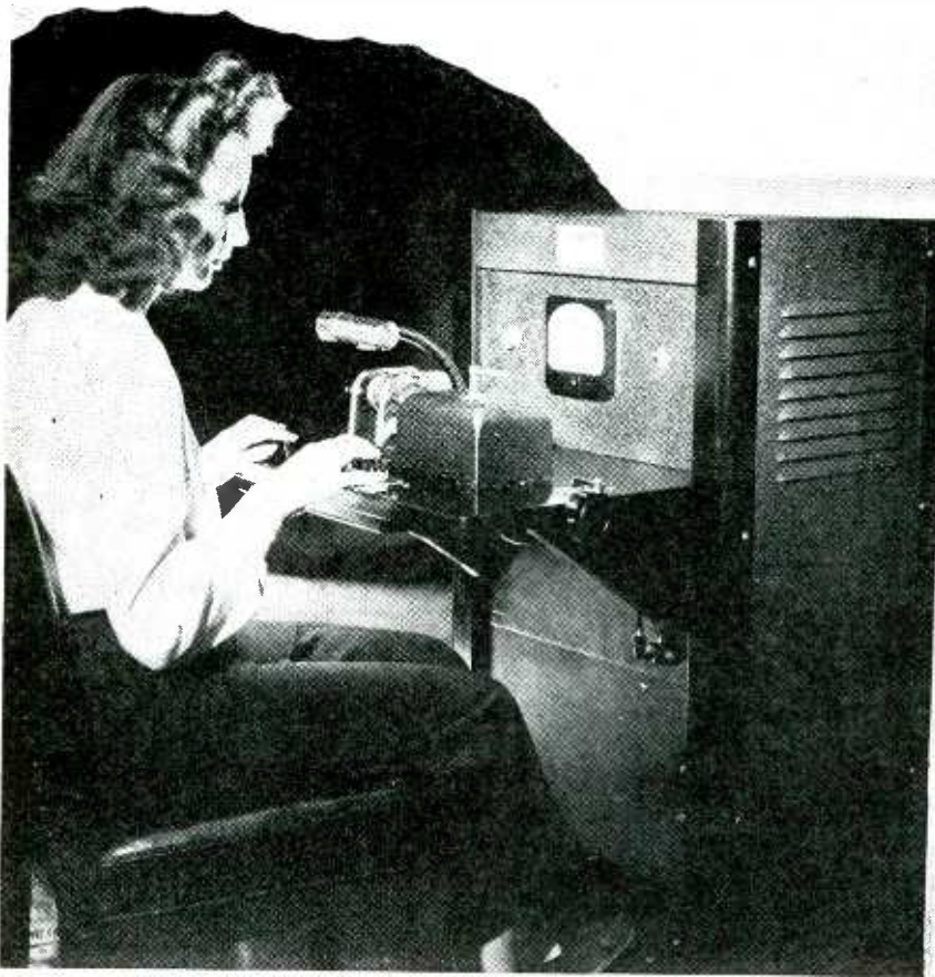
With this ultraprecision electronic balancing machine, a skilled operator can easily balance 200 gyro rotors a day to an accuracy of a few micro-ounce-inches. A drill press is conveniently located alongside the machine, and the operator alternately measures and drills until the required balance is achieved
